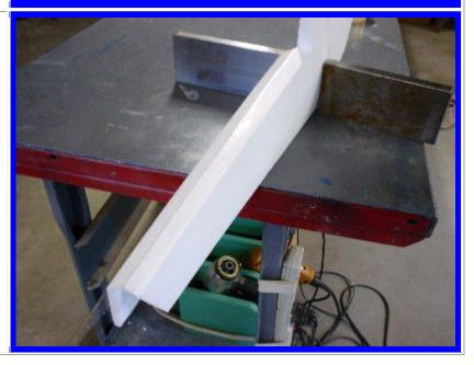
7. At this point the hinge is done. I have never seen a need for the two tape strips to touch at the hinge, although this works best for others. Notice that the aileron will be somewhat stiff in movement and it will not be in its neutral position. This doesn't matter once the servo and pushrod is in place.
