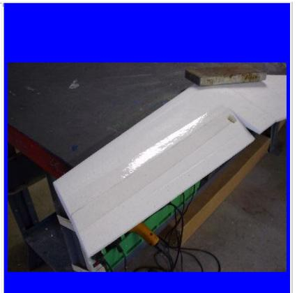
6. Then I stand the wing up (I use steel blocks to help hold it) and apply tape to the bottom of the hinge line, again half on the aileron and half on the wing. Burnish the tape down and trim the edges.
